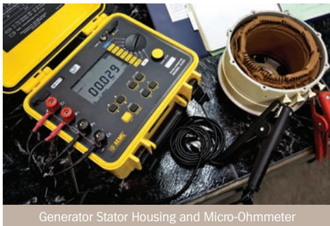
Generator Stator Housing and Micro-Ohmmeter
