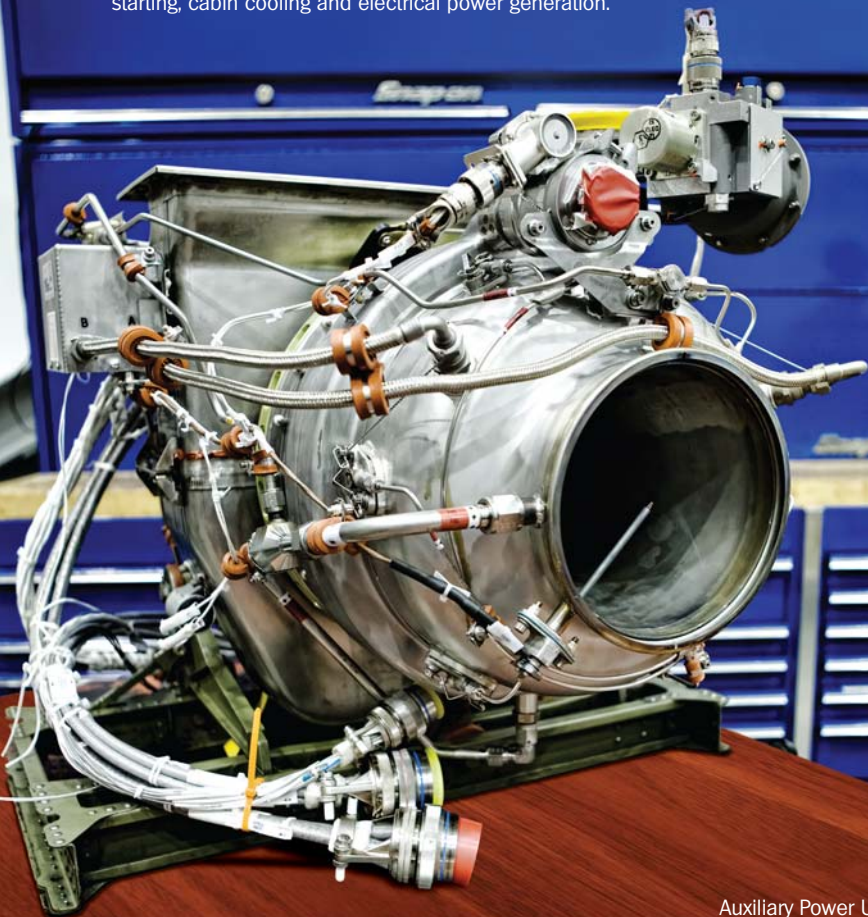
Auxiliary Power Unit
